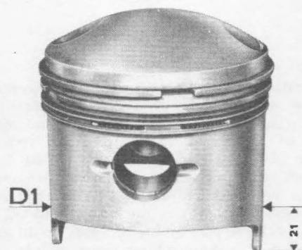
Piston diameter checking points
