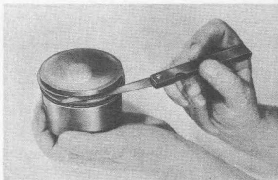
Checking vertical clearance
